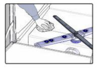
Now wipe the inside of the wash chamber ensuring any debris are removed and the chamber is clean, now reassemble all filters and wash arms.
